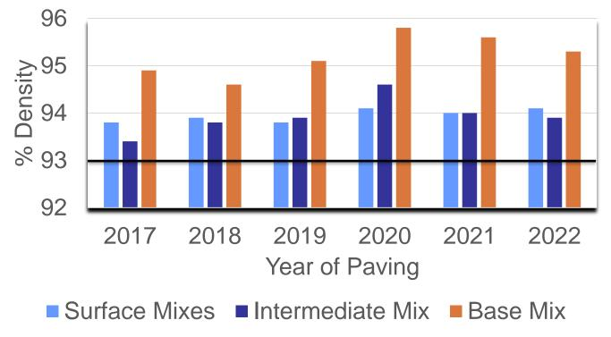
Spec Limit: 92.5% minimum density for SM, IM, and BM mixes
